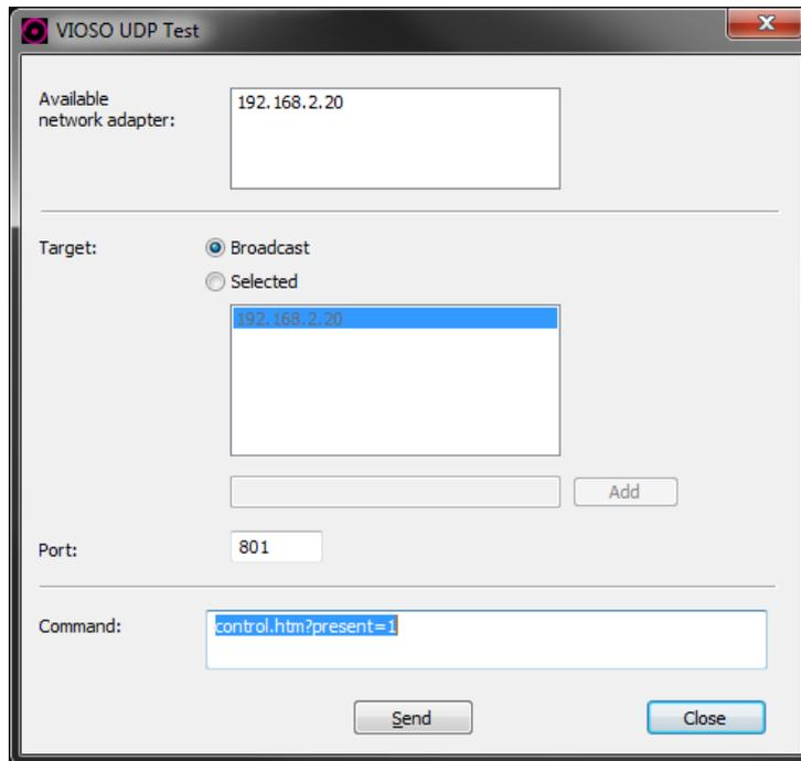
You can specify one or more targets by adding the IP of a desired PC to the target list. Beside this option, the tool is able to send the command string as broadcast to all computers in network.
