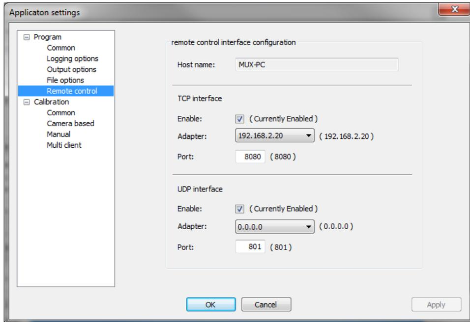
You must enable the desired interface type first. Then you should configure the network adapter and port to use. The special adapter ip 0.0.0.0 represents all available network adapter of used pc. After an restart of the application, the configured interface is available.
