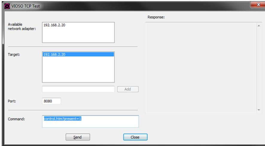
This tool does the same actions as its successor TCP Test Tool 2, but does not use a permanent connection and does not monitor all network traffic. It just outputs the response of the target.
